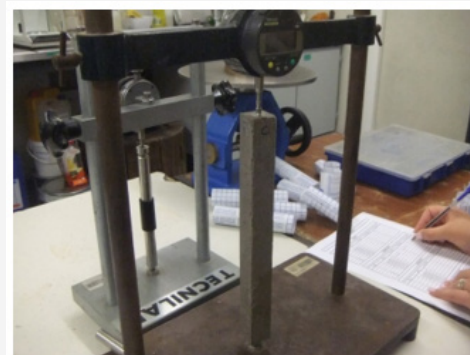
Figure 5: Shrinkage test: a) verifying the readings of the length comparator with the calibration rod; b) specimen measurements.
