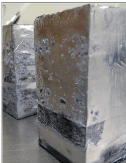
Figure 13: General view of a specimen soaked for 24 hours.
