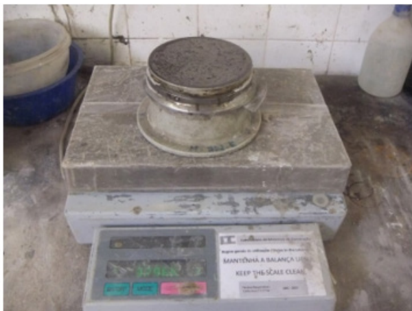
Figure 3: Determination of the bulk density of fresh mixtures, after vibration of the paste inside the bowl.
