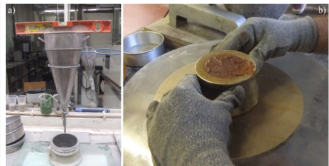
Figure 7: Fluidity analyses: a) set up of flow cone test; b) flow table test.
