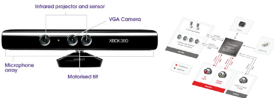
Figure 2.7: Kinect device and chip Cruz (2012)
