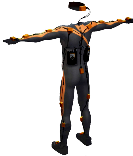
Figure 2.3: Human motion tracking system using inertial and magnetic sensors Roetenberg et al. (2009)
