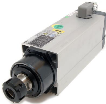
Figura 4.9: Motor spindle com bucha (HSD Mechatronics).
