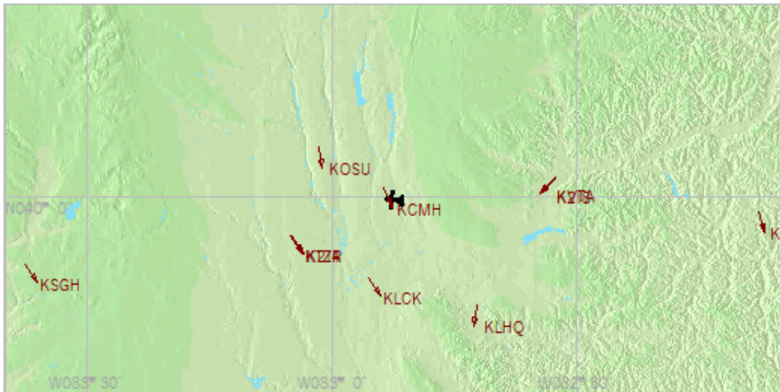
Figure 5.4: FSX's Weather Stations and Wind Information. The airplane denotes the spawn point for the player's airplane. In brown, there's the ICAO codes for available weather stations and, next to them, an arrow with the wind direction reported there.
