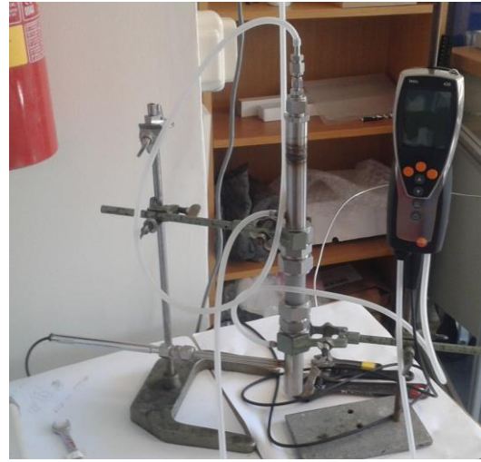
Figure 6 - Experimental installation for the pressure drop measurement
