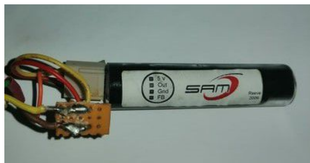
Figure 2.8: SAM Magnetometer that is used at IGUP. This is only one of three sensors i.e. it represents only one component of measurement.
