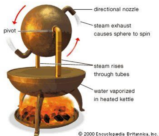
Figure 2 - Schematic of an Aelolipile (Encyclopaedia Britannica, 2000)
