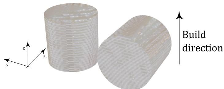
Figure 2.2: Schematic representation of same cylinder design printed with two distinct orientations.
