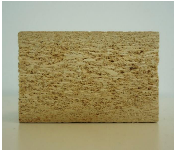
Figure 1.9. Internal section of particleboard made from Populus spp. wood.
