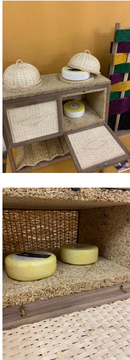
Figure A.2. Sideboard for cheese and wine produced with a cardoon particles and a potato starch-based adhesive. The panels were pressed at 16 mm during 60 s, then the top platen was raised at 25 mm and the panel was maintained in the press during 240 s. The temperature of press platens was 190 °C. This piece of furniture was on display in London Design Fair and Salone del Mobile Milano.
