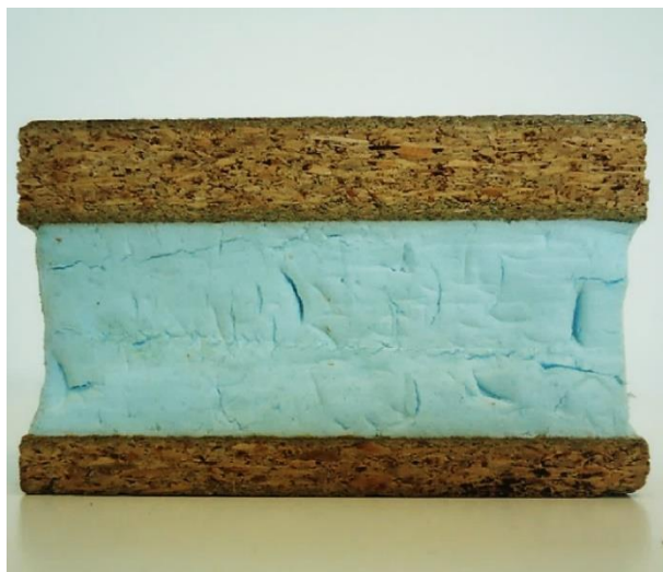
Figure 1.14. Sandwich panel with a polystyrene foam core and wood-based particleboard in the facings.
