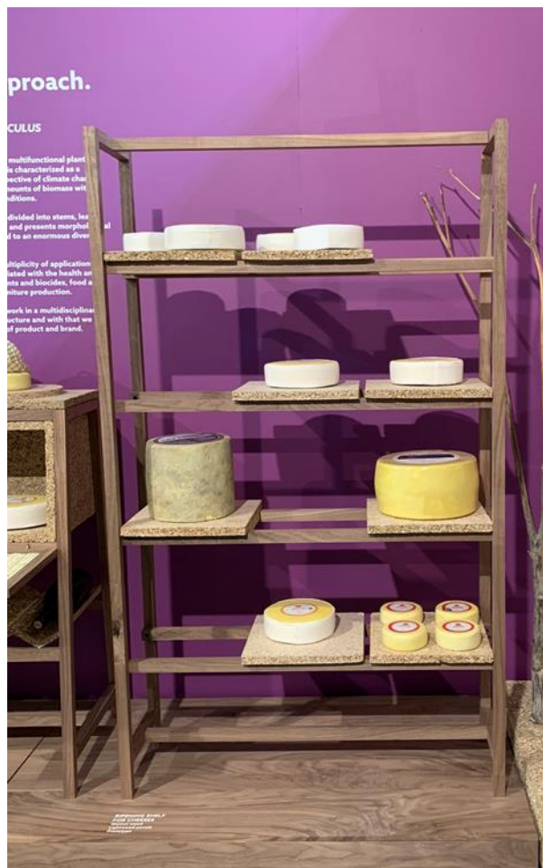
Figure A.1. Shelves for cheese ripening produced with a cardoon particles and a potato starch-based adhesive. The panels were pressed at 16 mm during 60 s, then the top platen was raised at 25 mm and the panel was maintained in the press during 240 s. The temperature of press platens was 190 °C. This piece of furniture was on display in London Design Fair and Salone del Mobile Milano 2019.
