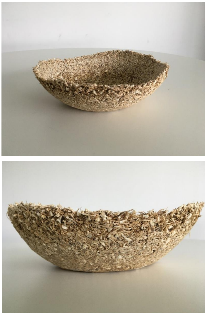
Figure A.3. Fruit bowl produced with a cardoon particles and potato starch-based adhesive. The piece was produced at 190 °C using a mould.
