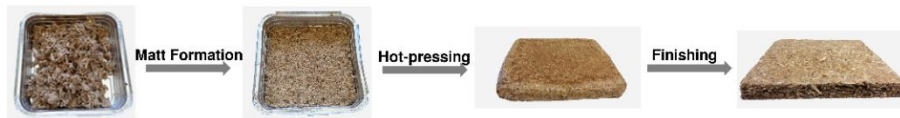
Figure 3.1. Steps of manufacture process of particleboards bonded with a sour cassava starch, starting with a mixture of wood particles and starch paste and ending with a finished particleboard.
