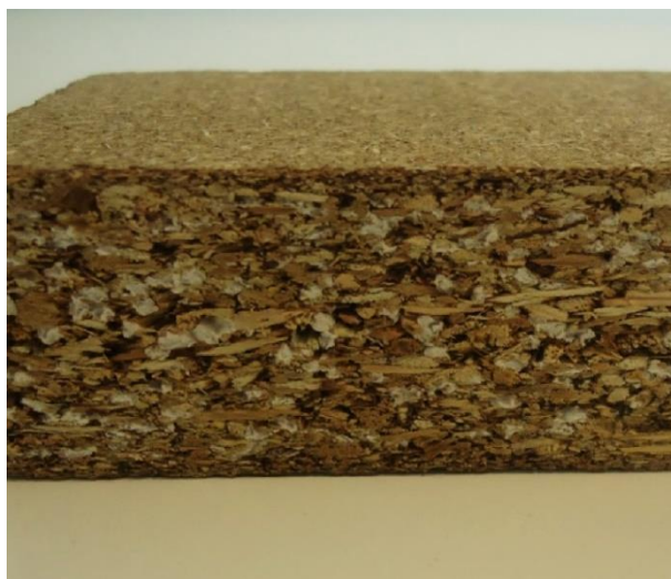
Figure 1.10. Internal section of particleboard produced with expanded polystyrene foam (EPS) mixed with wood particles in core layer.
