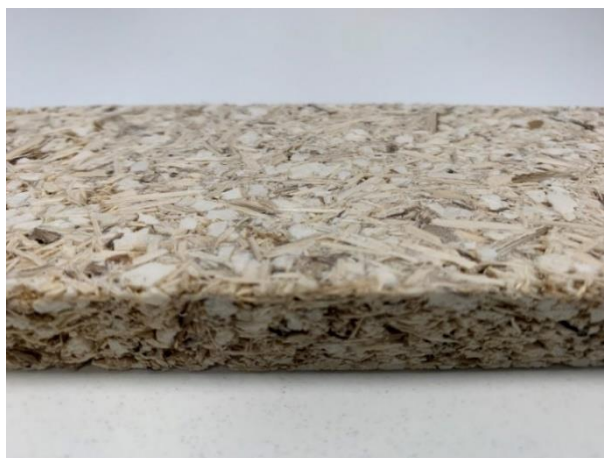
Figure 4.14. Cardoon particleboard with potato starch binder. Panel thickness is 16 mm.
