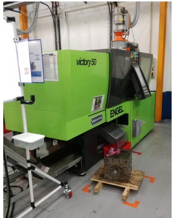
Figure 38 New Border of line - All materials close to the operator, more ergonomic workplace, quality control stand in front of operator.
