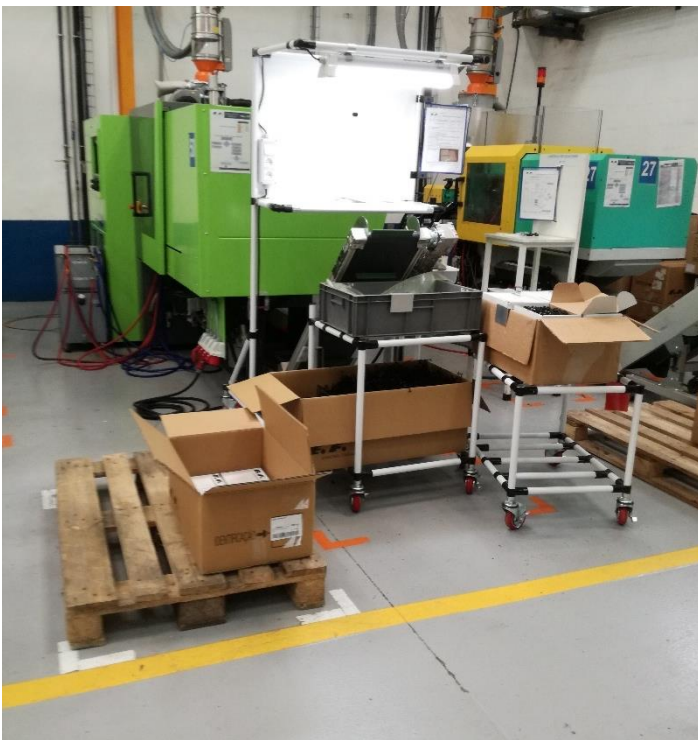
Figure 38 New Border of line - All materials close to the operator, more ergonomic workplace, quality control stand in front of operator.
