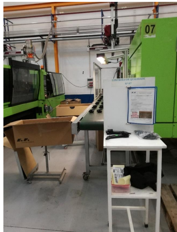
Figure 37 Initial Situation - Disorganized workplace, no standardized border of line, quality control far from operator
