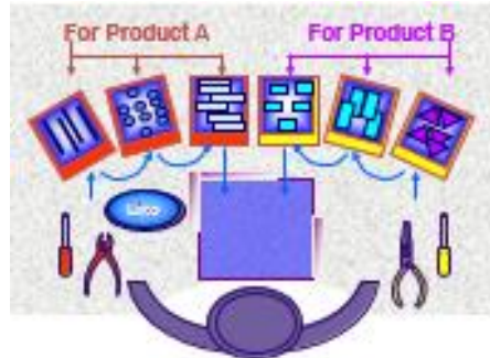
Figure 6 A correct border of line: 5s applied and materials are in small, easy to reach packages
