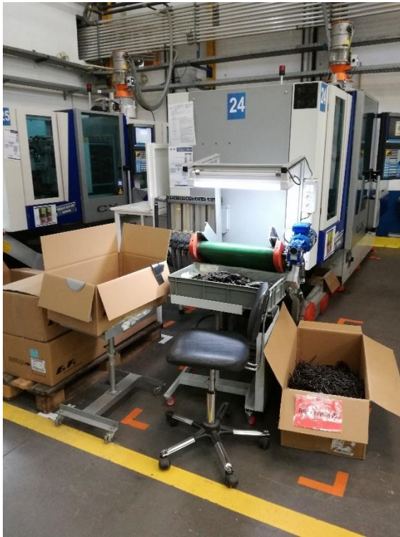
Figure 37 Initial Situation - Disorganized workplace, no standardized border of line, quality control far from operator
