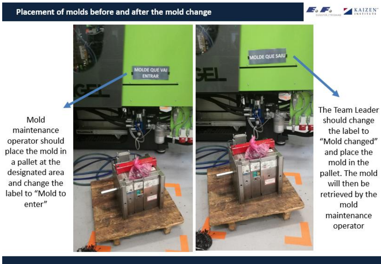
Figure 39 Visual Norm: mold placement before and after change
