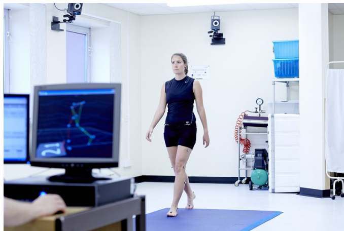
Figure 2.16: Example of the gait analysis performed by a camera based system with markers (HS) (VICON gait analysis 22 ).
