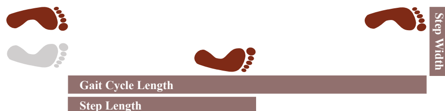
Figure 2.5: Spatial Parameters: GC length (stride length), step length and step width.
