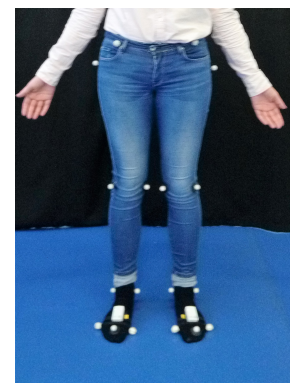
(d) Markers placed at the lower limb. View from the anterior part. Without the femur and tibia markers. With SWORD Health's sensors system.
