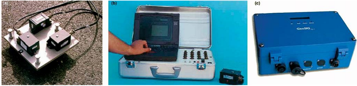
Figure 30 - (a) Force balance accelerometers; (b) multichannel data acquisition and processing system for ambient vibration tests; (c) strong motion triaxial seismograph
