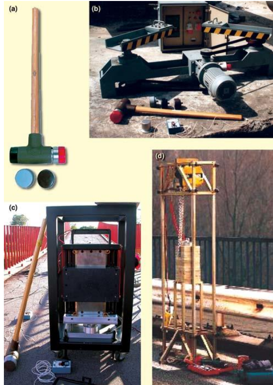
Figure 28 - (a) Impulse hammer; (b) eccentric mass vibrator; (c) electrodynamic shaker over three load cells; (d) impulse excitation device for bridges.
