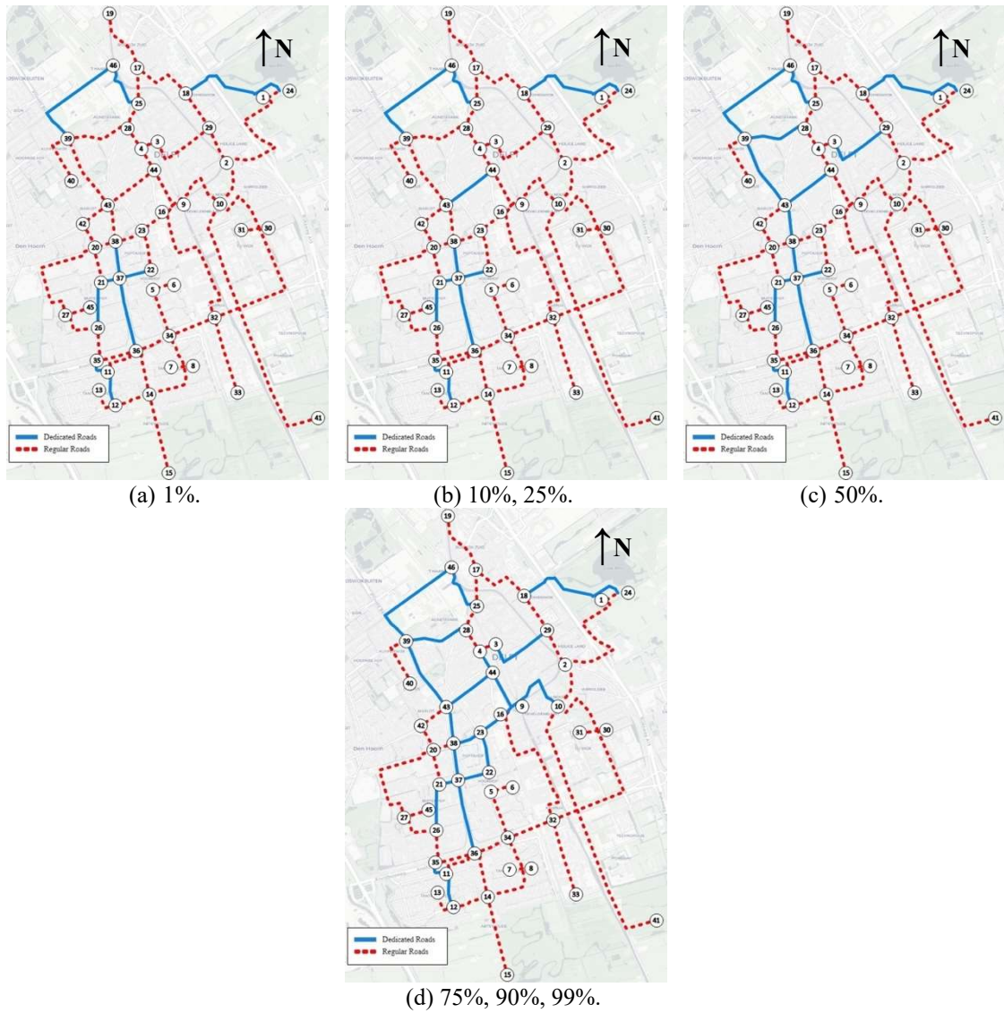
Figure 3.6 – RNDP-AVs peak-hour design: AV subnetworks of Scenario I under Incremental Planning (a), (b), (c), and (d) (% of AV penetration rate).
