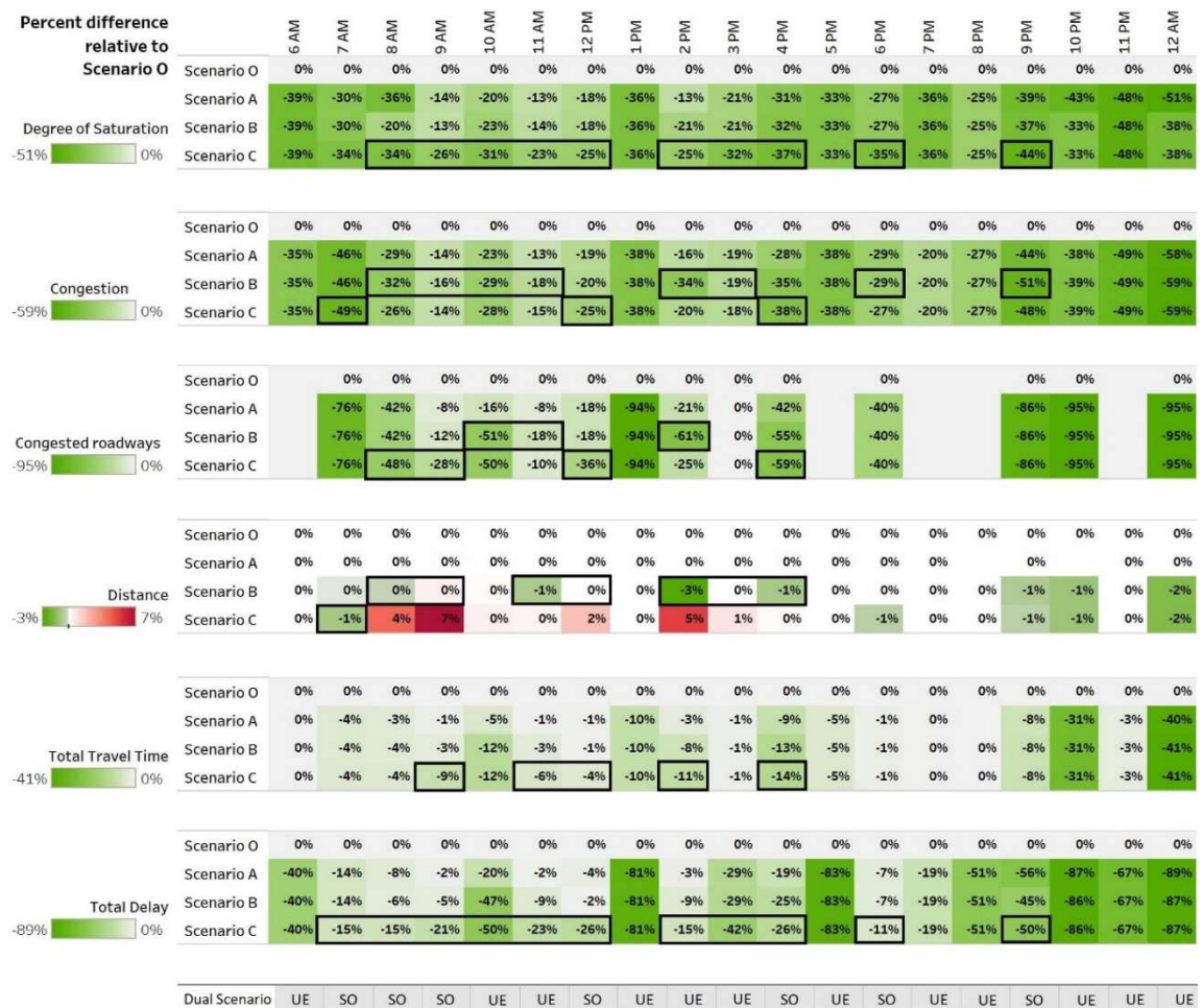
Figure 4.10 – Hourly analysis of the main traffic performance indicators (Conceição et al., 2020).
