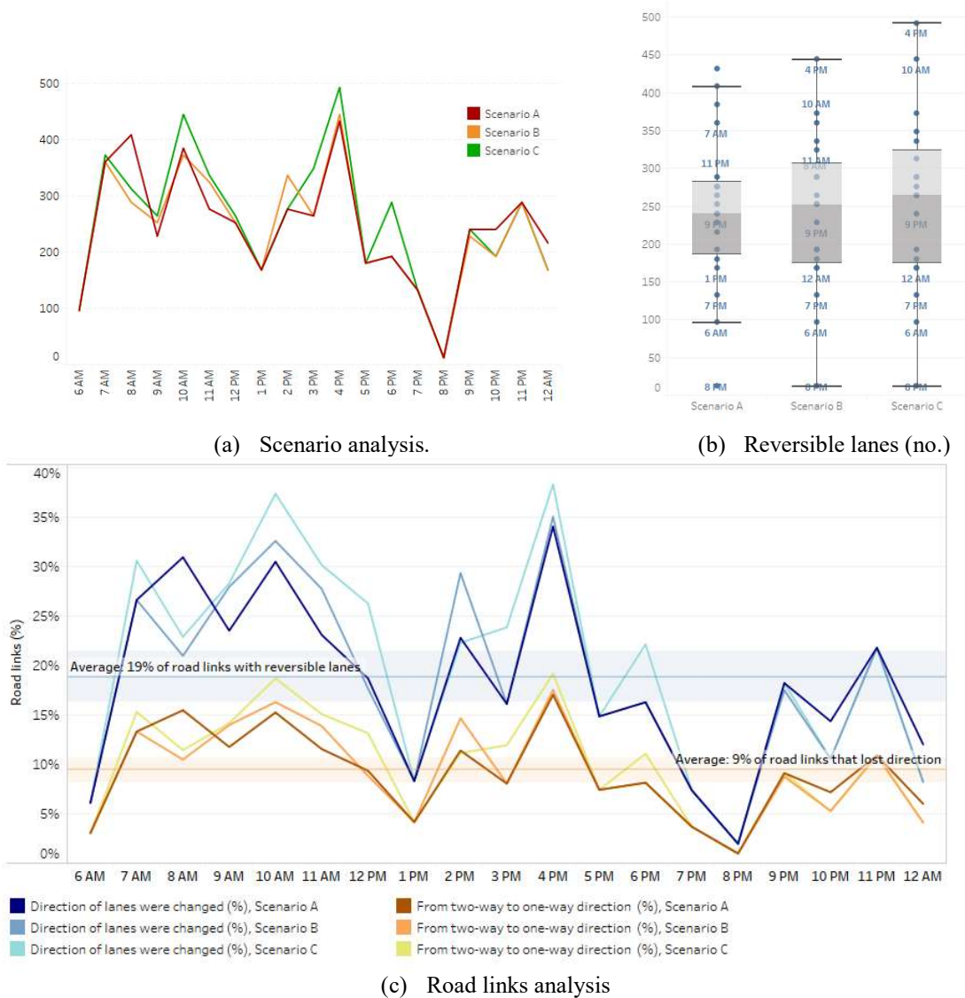
Figure 4.3 – Graphical analysis of the reversible lanes strategy throughout the day: (a) Scenario analysis; (b) number of reversible lanes; (c) Road link analysis.
