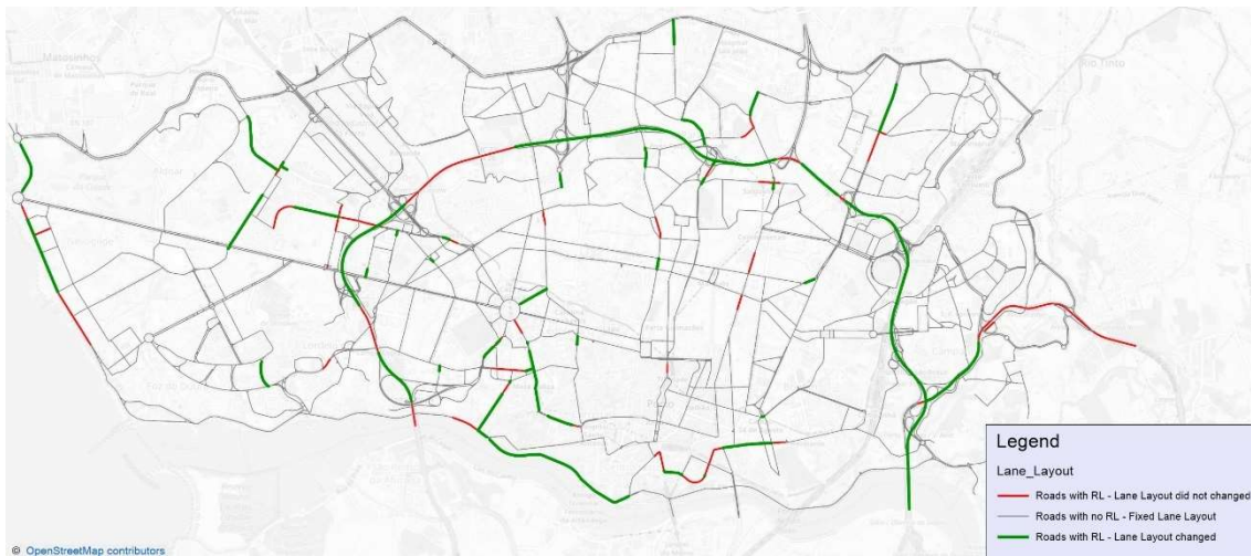
Figure 5.20 – Lane layout of the RL-NDP_SOF experiment II of the Porto case study (VISUM).
