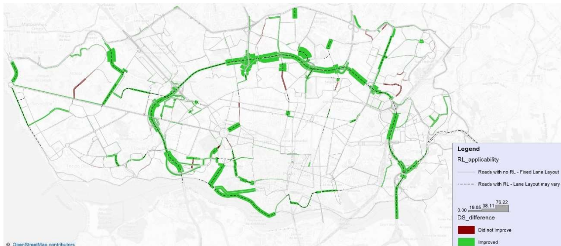
Figure 5.21 – Analysis of the traffic improvement in terms of the degree of saturation in the RL-NDP_SOF experiment II of the Porto case study (VISUM).
