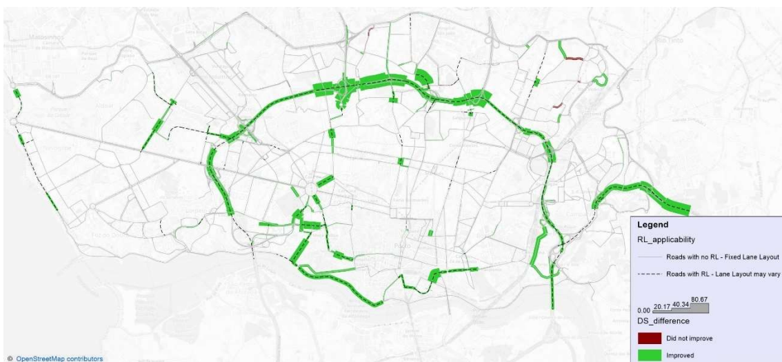
Figure 5.15 – Analysis of the traffic improvement in terms of the degree of saturation in the RL-NDP_SOF experiment I of the Porto case study (VISUM).
