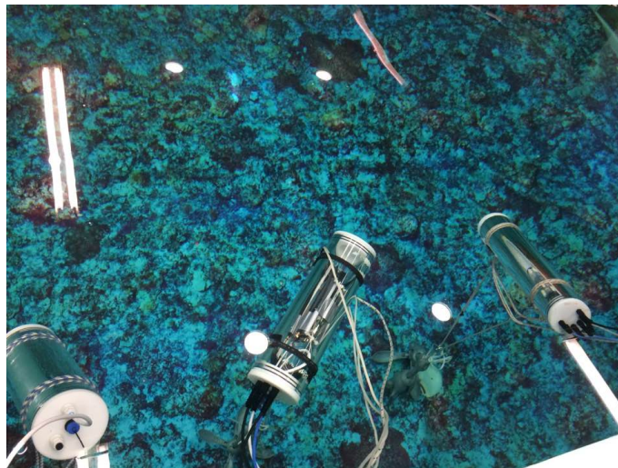
Figure 6.3: Testbed for data mule experiments between sender and receiver nodes in INESC TEC
