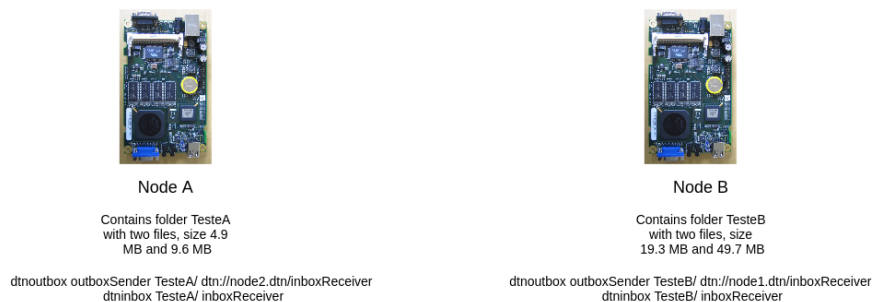
Figure 3.18: Procedure applied in testing bidirectional file transfer with dtininbox and dtnoutbox
