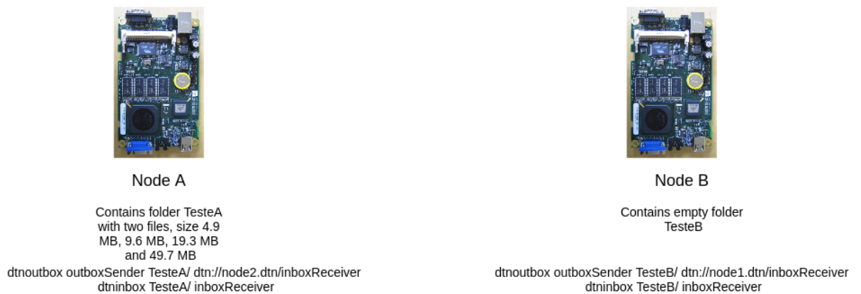
Figure 3.16: Procedure applied in testing one way folder transfer using dtinibox and dtnoutbox simultaneously
