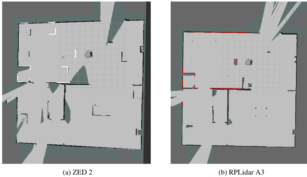
Figure 6.9: Resulting maps using the ZED 2 and RPLidar sensors respectively.
