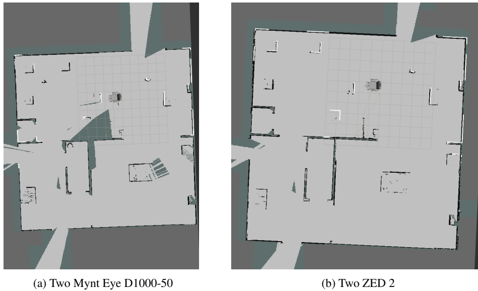
Figure 6.11: Resulting map of using two Mynt Eye D1000-50 and two ZED 2 respectively.
