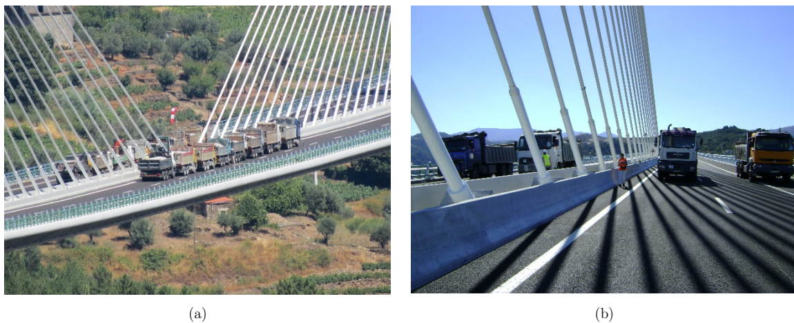
Figure 3.11 – Position of the vehicles during the load case CC14 (a) and during the crossing for obtaining the centred influence line.
