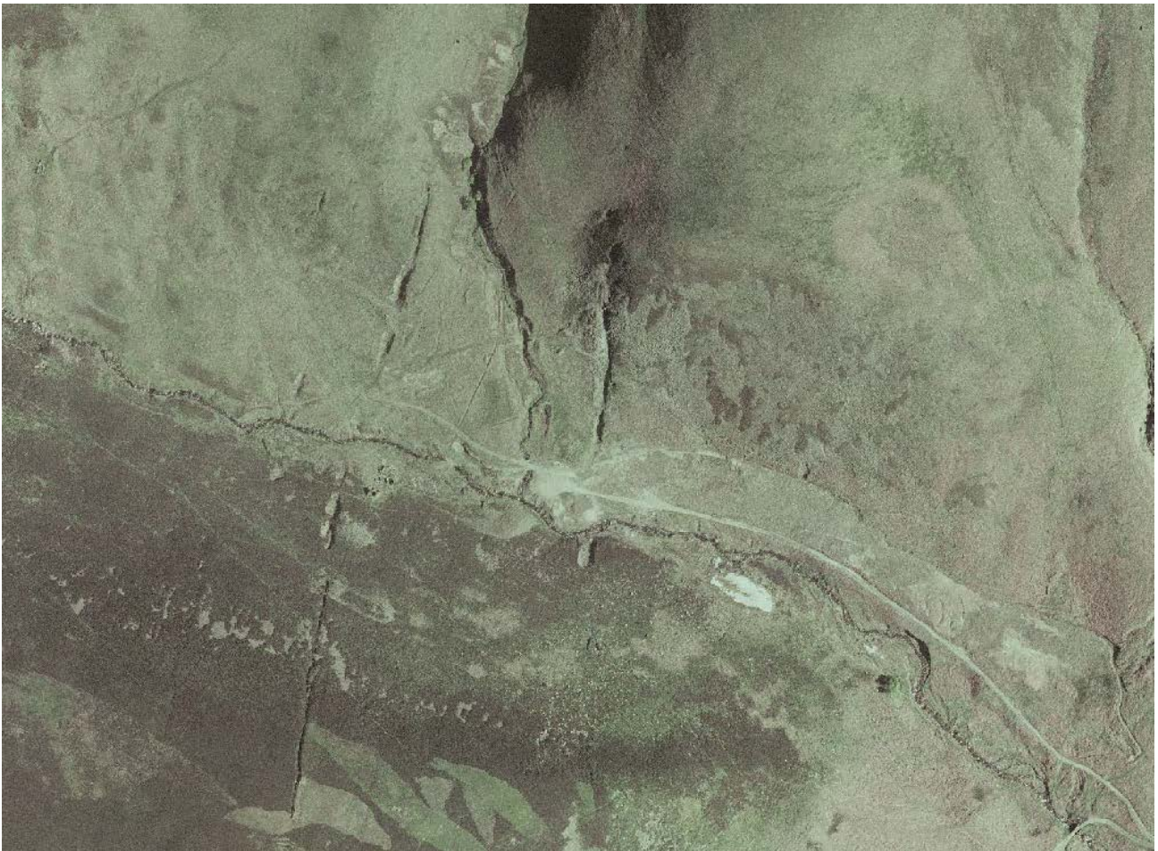
Figure 1: Aerial photograph of the Carrock Mine site. Note the long line of surface workings on Harding Vein (west of centre) with two smaller surface workings further west on Smith Vein and those on Emerson Vein in the centre, east of Brandy Gill Beck. The mill was in the centre of the image (NE of the confluence of Brandy Gill Beck with Graingill Beck and tailings of various vintages can be seen at the mill site and to the east both south of Graingill Beck (white) and north of the mine access road (red-brown). Width of image approximately 825m. Aerial photography ©UKP/Getmapping Licence No. UKP2006/01.
