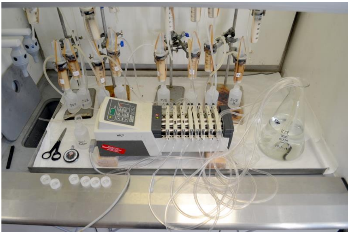
Plate 4 Elution in progress, with the samples are being collected in 125 ml nalgene™ bottles
