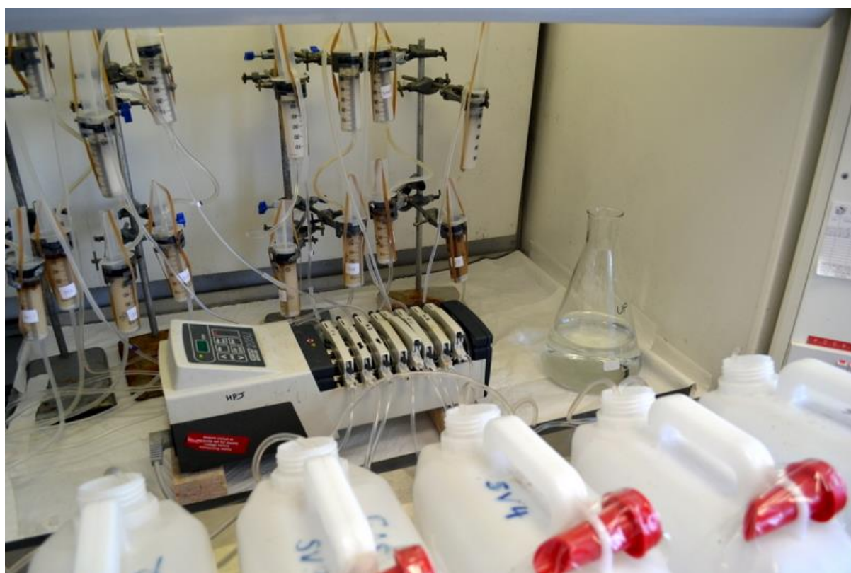
Plate 3 Samples being pumped through the resin column by a peristaltic pump
