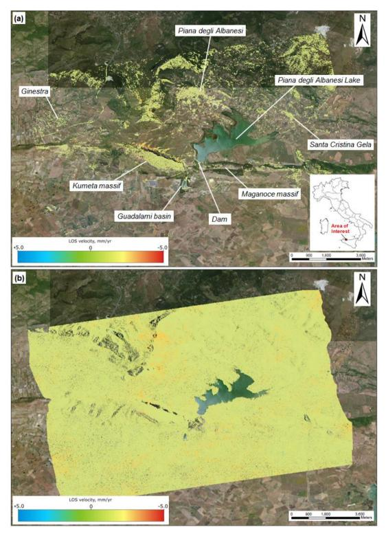
Figure 1: Annual ground motion rates for the area of Piana degli Albanesi (Italy), obtained from the (a) SBAS and (b) ISBAS processing of COSMO-SkyMed StripMap HIMAGE ascending mode data acquired between 2008 and 2011. Motion velocities are saturated to ±5.0 mm/yr. SBAS and ISBAS results are overlapped onto World Imagery [Source: Esri, DigitalGlobe, GeoEye, i-cubed, Earthstar Geographics, CNES/Airbus DS, USDA, USGS, AEX, Getmapping, Aerogrid, IGN, IGP, swisstopo, and the GIS User Community].
