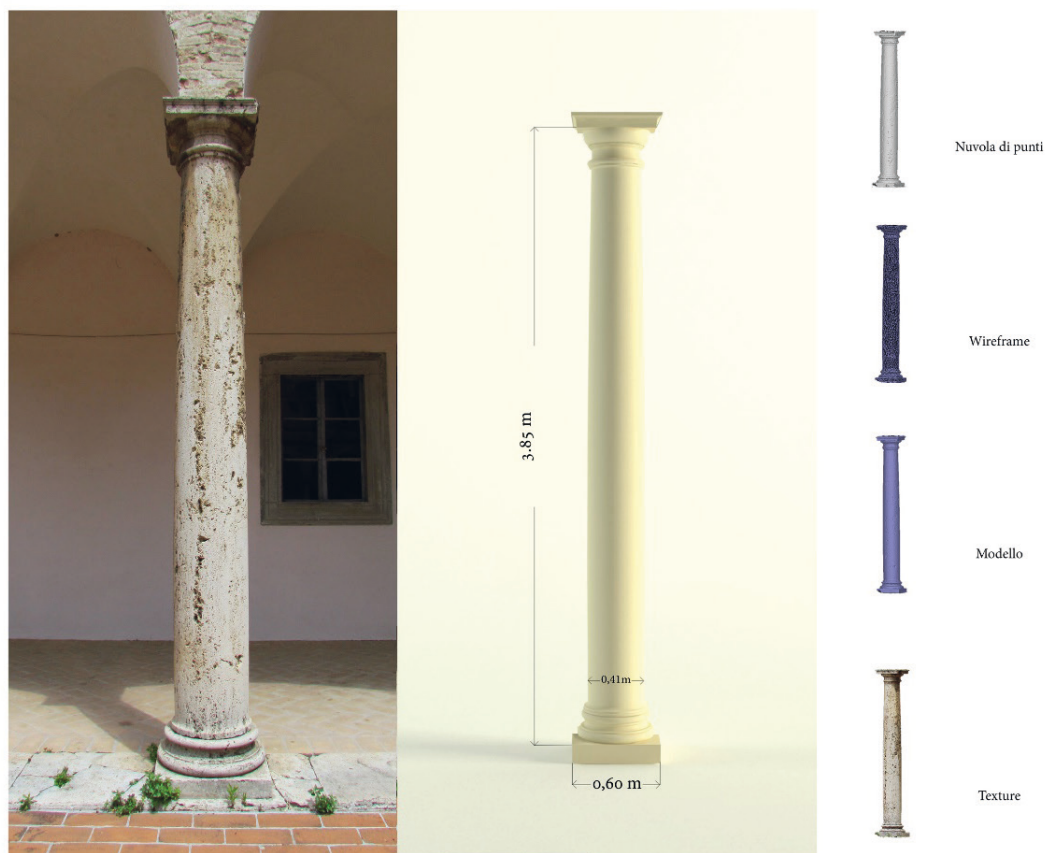
Figure 5. The Doric column modelling.
