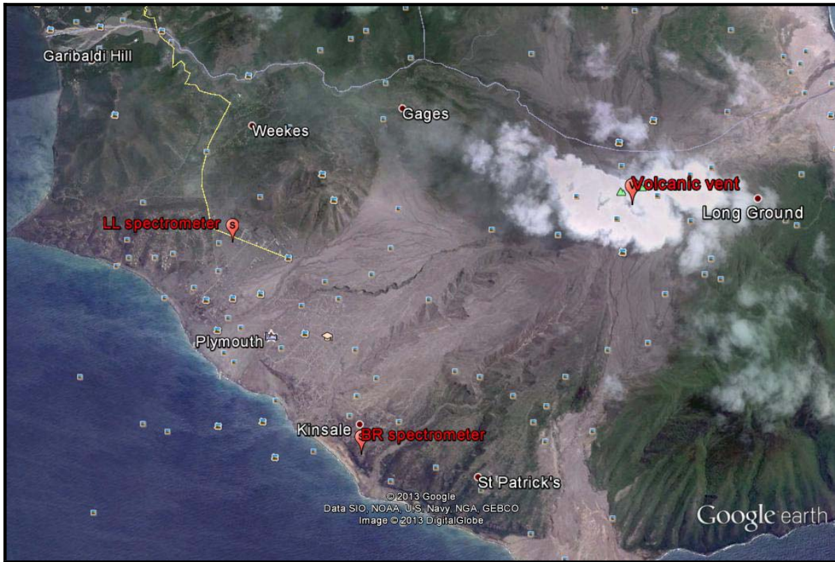
Figure 2 Google Earth image of southern Montserrat showing the location of the two network spectrometers relative to the volcano. The spectrometers are named based on their location (LL – Lovers lane, BR – Brodericks) . The prevailing winds are easterlies which normally puts the plume over Plymouth. In this image the plume is to the north of the network.
