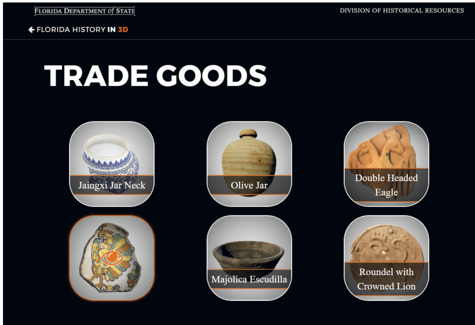
Figure 9. The galleries, in this case the one on trade goods, were generated dynamically on the server from a JSON array of model IDs.
