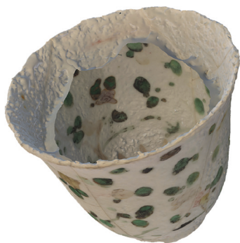
Figure 3. One attempt at a porcelain cup produced a pockmarked, interior-free model due to the impact of surface reflection on the modelling process.
