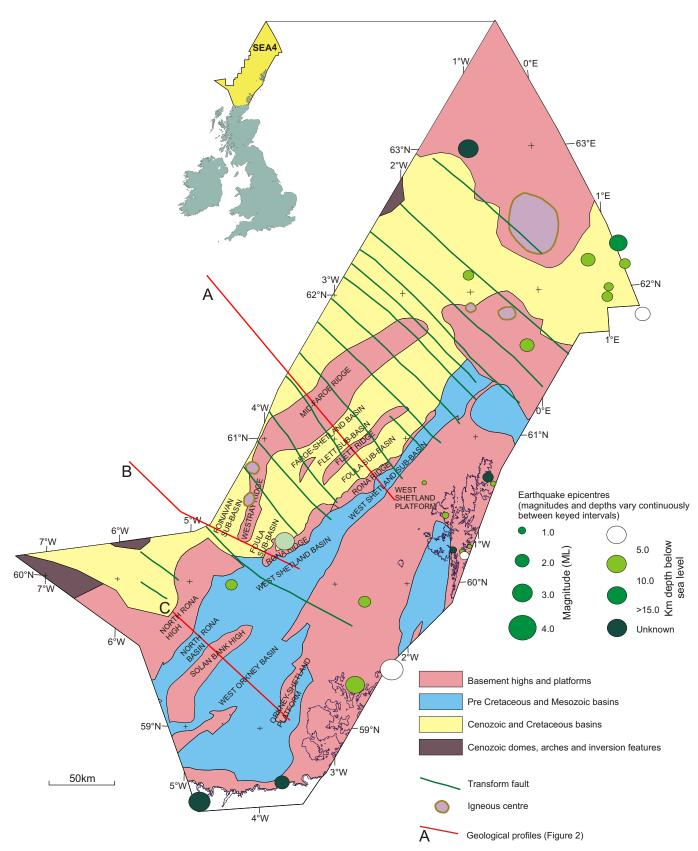
**Figure 1 Generalised structural geological framework and natural seismicity** Structure adapted from BGS Passive Margins Modelling Project (Gatliff, *pers comm.*2003). The inset map shows a complex boundary to the NW limits of data in SEA4 and this boundary has been excluded for purposes of clarity.
