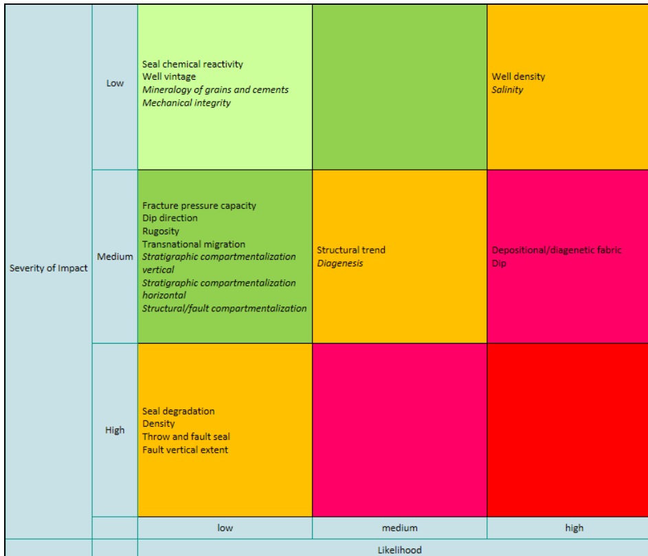
Fig. 6. Containment and operational risk factors with an effect on storage capacity for storage unit 139.016 (operational risks in italics).
