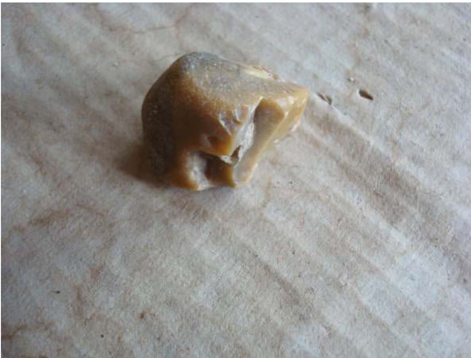
Figure 4: Slightly abraded, broken, sub-rounded, oxidised flint pebble from 35 m depth.
