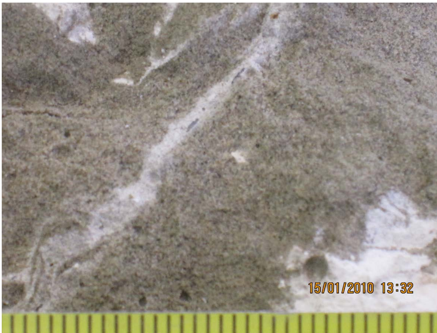
Figure 3: Close-up of chalky smear in centre of Figure 4 with tiny angular flint shards, depth of 41 m. Scale in millimetres.
