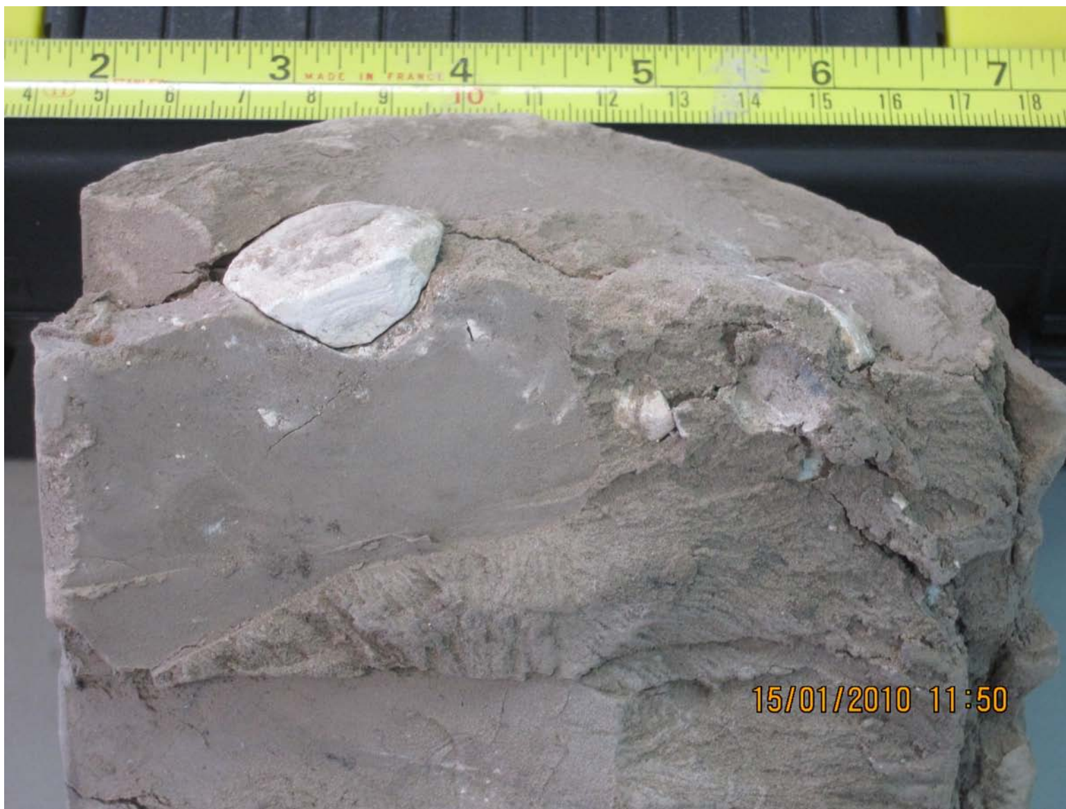
Figure 5: ‘Alluvium’: Layer of calcareous clasts in weakly laminated silty clay, depth of 17.33 m.
