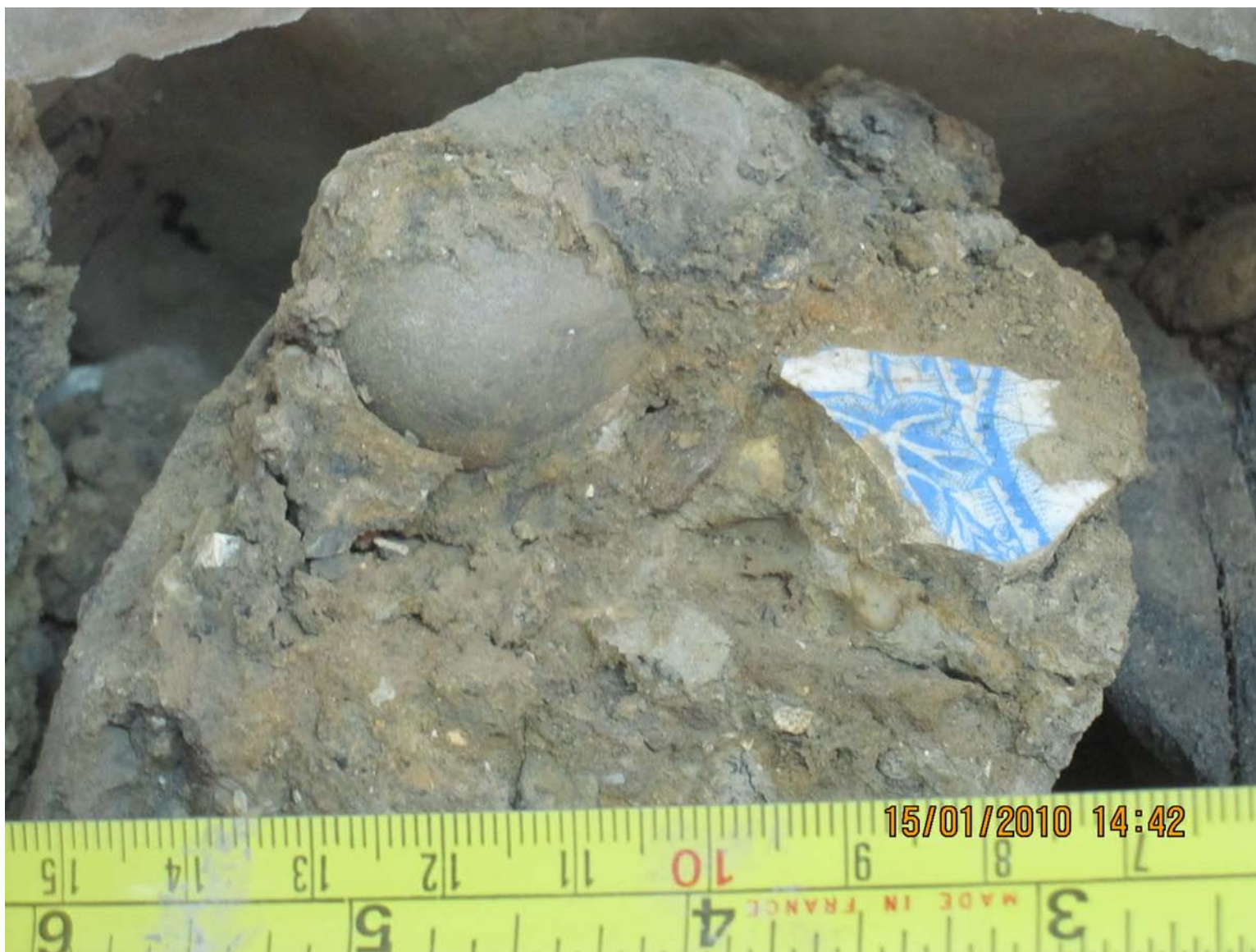
Figure 6: Made ground: clayey sandy gravel with fragment of glazed pottery from depth of 16.3 m.
