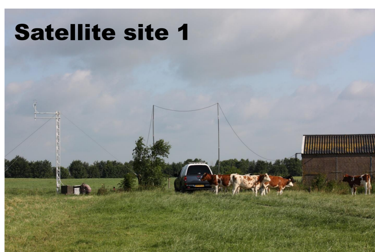
Satellite site 1 6 m height: METEK USA-1 + FMA gas analyser (Los Gatos Research)
