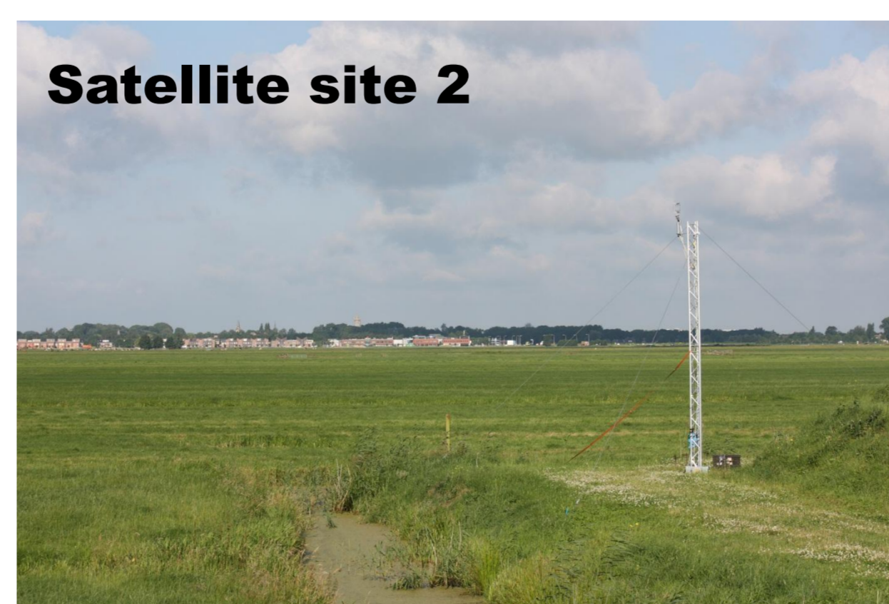
Satellite site 2 6 m height: Gill Windmaster Pro + DLT-100 gas analyser (Los Gatos Research)
