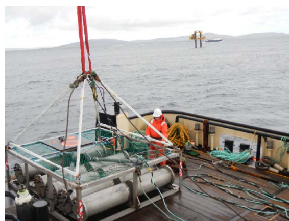
Figure 1. The FLOWBEC frame about to be deployed at the EMEC tidal site
