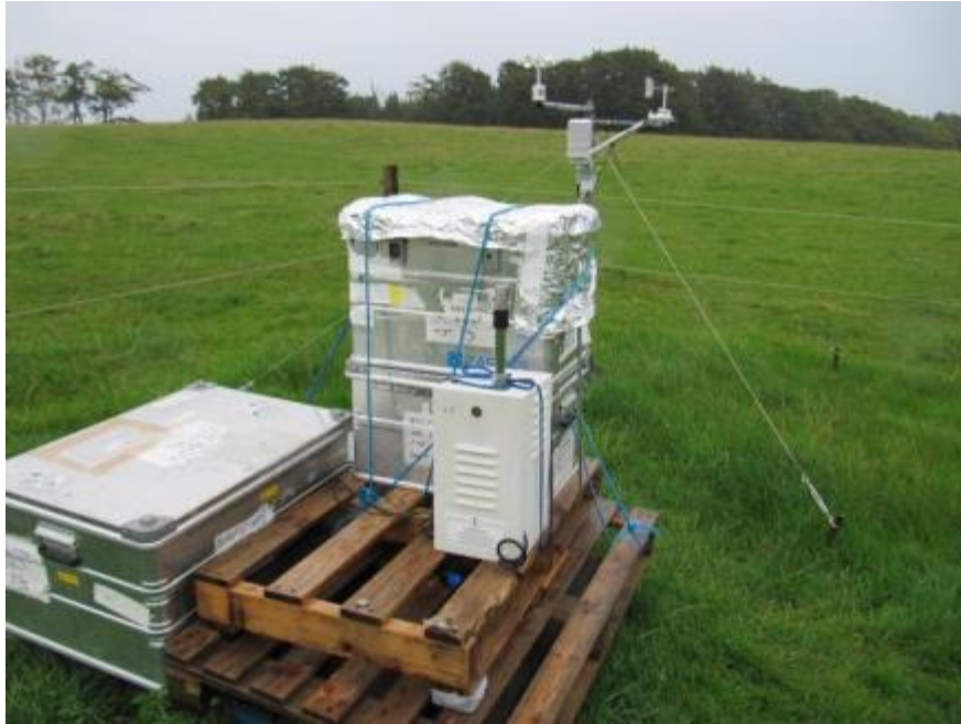
Figure 14: Osiris monitor deployed in the field in a weather proof enclosure at Whitelees farm (site White 1).
