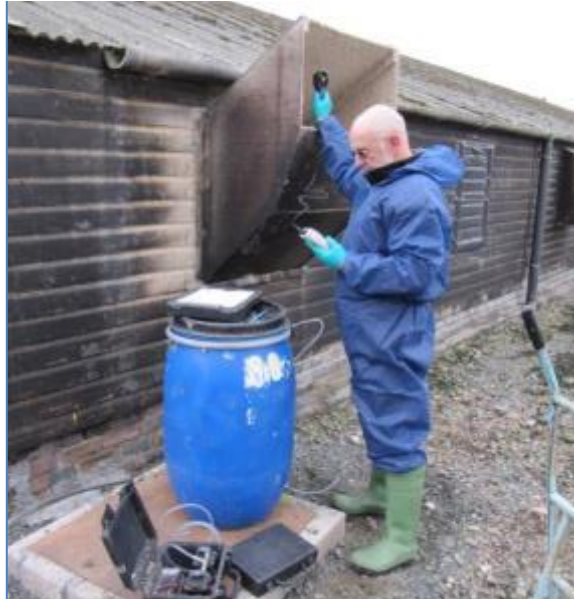
Figure 8: Monitoring odour concentrations and fan ventilation flows in the exhaust of Glendevon farm.
