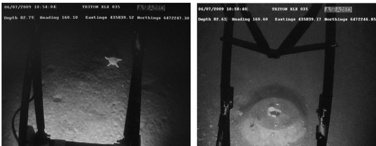
Figure 10.13 Images extracted from the ROV video, showing a starfish and one of the concrete gravimetry benchmarks on the seabed.
