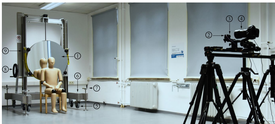
FIGURE 1 Schlieren imaging system at Bauhaus-Universität Weimar, see text for legend
