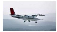
Airborne geophysical surveys require low altitude flying to acquire high resolution data on the subsurface. Image courtesy Tellus Border project, supported by the EU INTERREG IVA Cross-Border programme.
