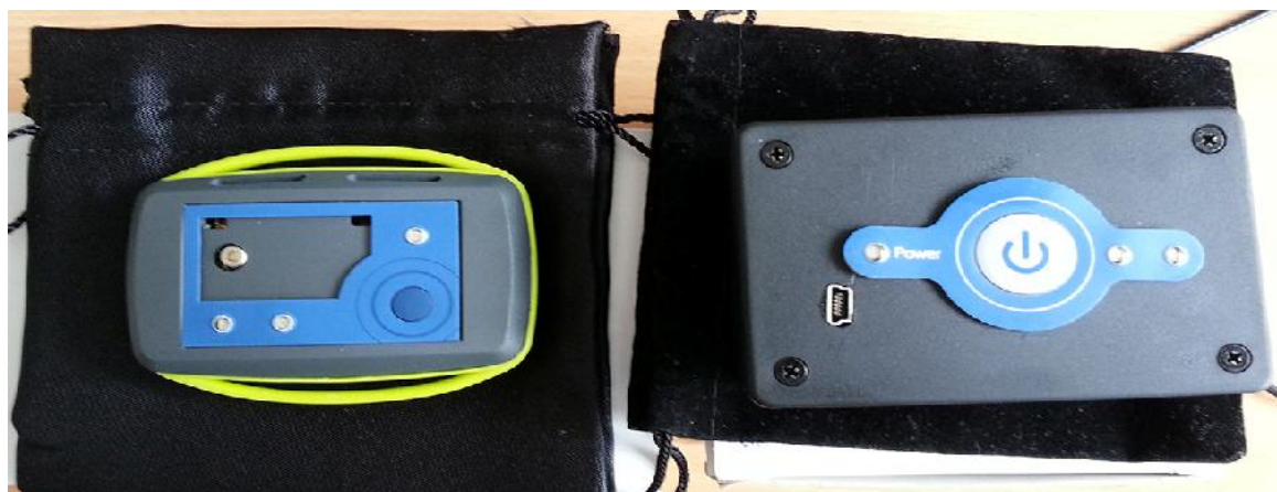
Figure 3.2. Sensaris EcoO3Sense (left) and EcoPM (right) sensors tested in April 2013 (Dimensions EcoO3 - 50 x 80 x 20 mm; EcoPM 75 x 97 x 46 mm (W x L x H))
