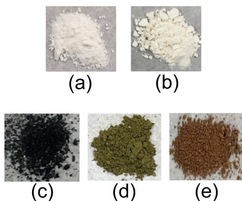
Figure 2. Optical photographs of products obtained after (a) hydrothermal treatment, (b) washing of (a) with aqueous solution of \text{HNO}_3 and deionized water, (c) calcination using (b) and urea at 930\text{ }^\circ\text{C} for 2 h, (d) calcination using (a) and urea at 930\text{ }^\circ\text{C} for 2 h, and (e) calcination using (b), commercial \text{La}(\text{OH})_3 and urea at 930\text{ }^\circ\text{C} for 2 h.
