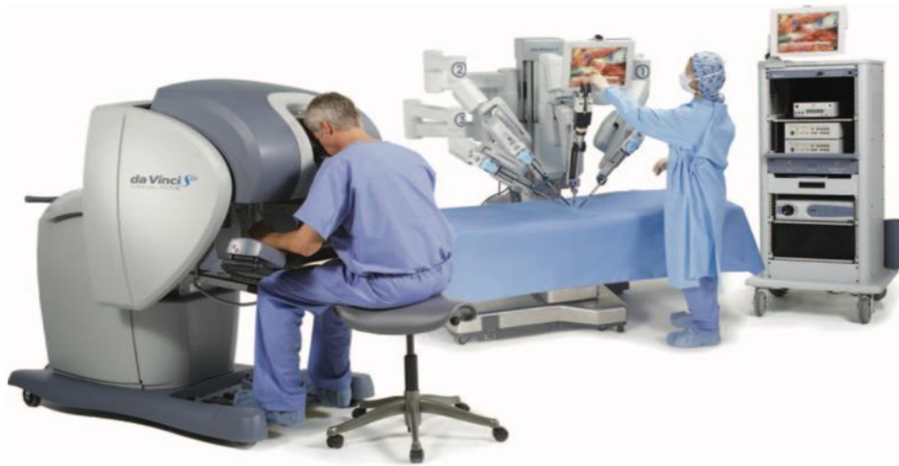
Figure 4 Da Vinci robotic systems have three major components: the surgeon console, the surgical cart, and the vision cart (Schreuder and Verheijen 2009, 200).
