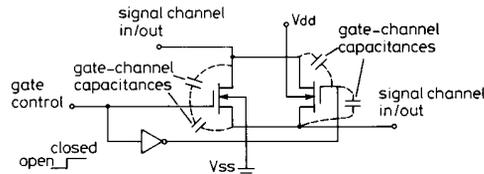
Fig. 3 Structure of CMOS switches
