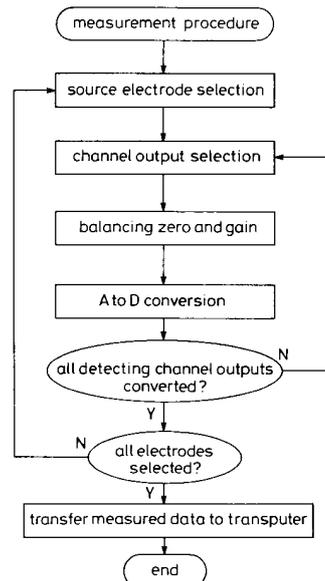
Fig. 6 Measurement procedure
