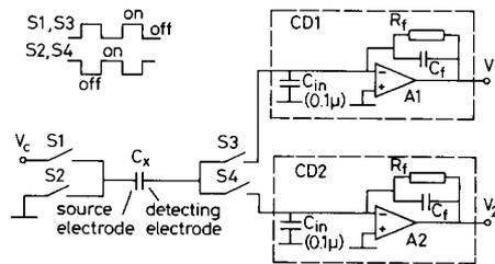
Fig. 2 Basic capacitance measurement circuit
