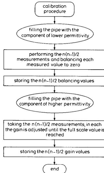
Fig. 5 Calibration procedure
