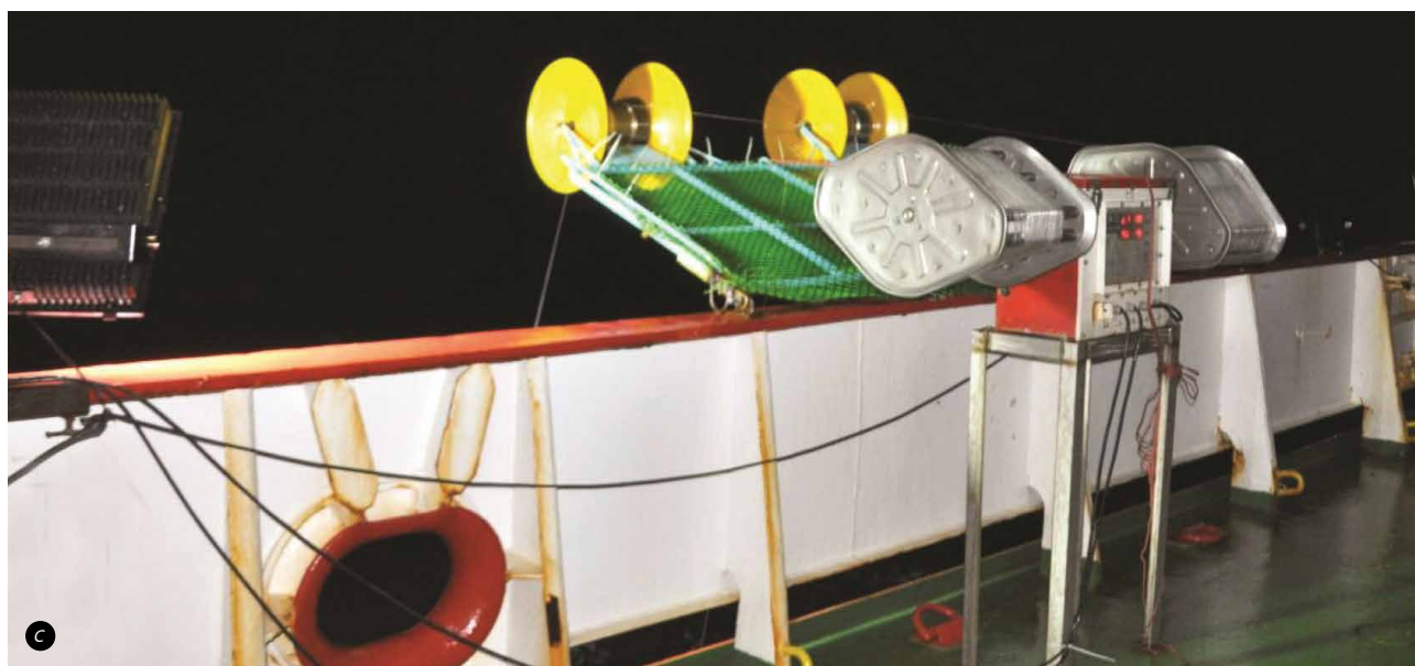
Fig. 2. Sampling operations during the 10 th and 11 th Indian expedition to Southern Ocean/ Antarctic waters (a) RMT (b) IKMT, for cephalopod paralarvae and juveniles; (c) Automatic squid jigging machine used for the capture of adult squids.
