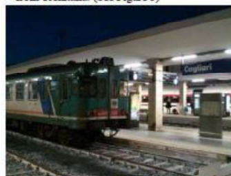
Figure 3 Diesel locomotive ALN 668-3114 from Trenitalia
