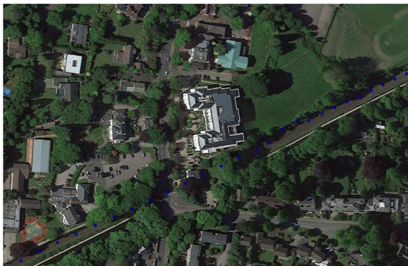
Figure 2.4 Example Kalman Filter Positioning for Real GPS Rail Data (EATS n.d.)
