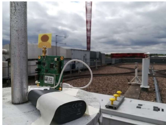
Figure 5.9 UWB anchor placement example
