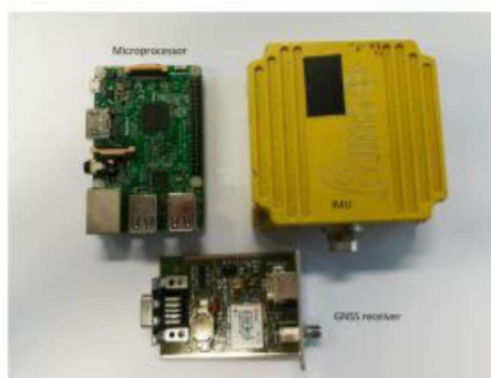
Fig. 1. Positioning and line characterization system hardware for the prototype implementation.
