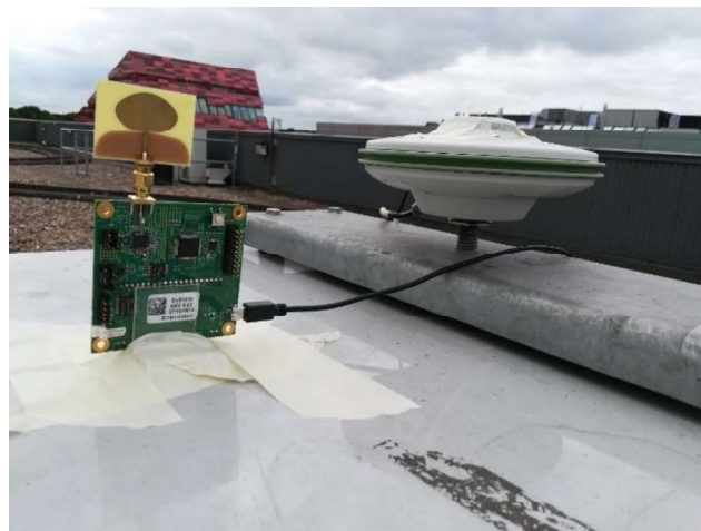
Figure 5.8 UWB Antenna placement
