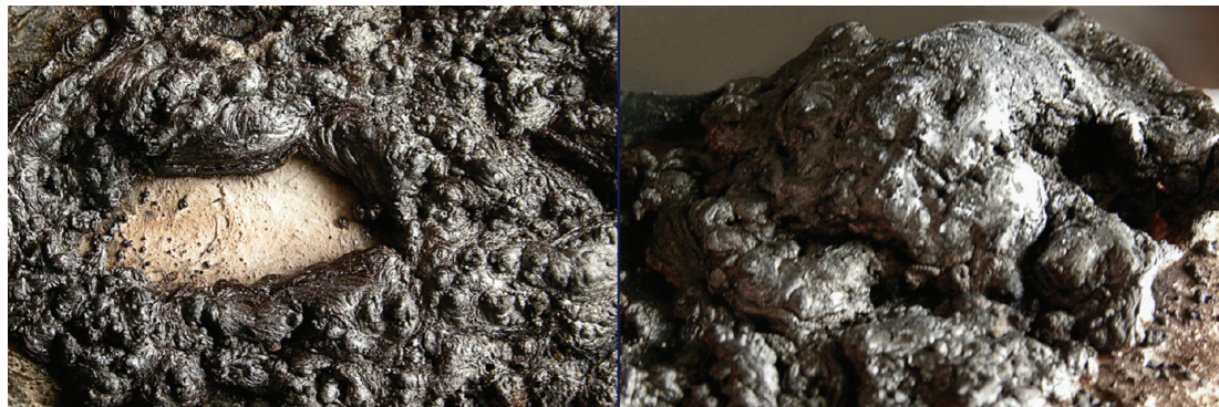
Figure 4. Performance of coating RII in the inclined tunnel: (left) slight depression attributable to the flame pressure; (right) between 28 and 30 mm height of the intumescence.
