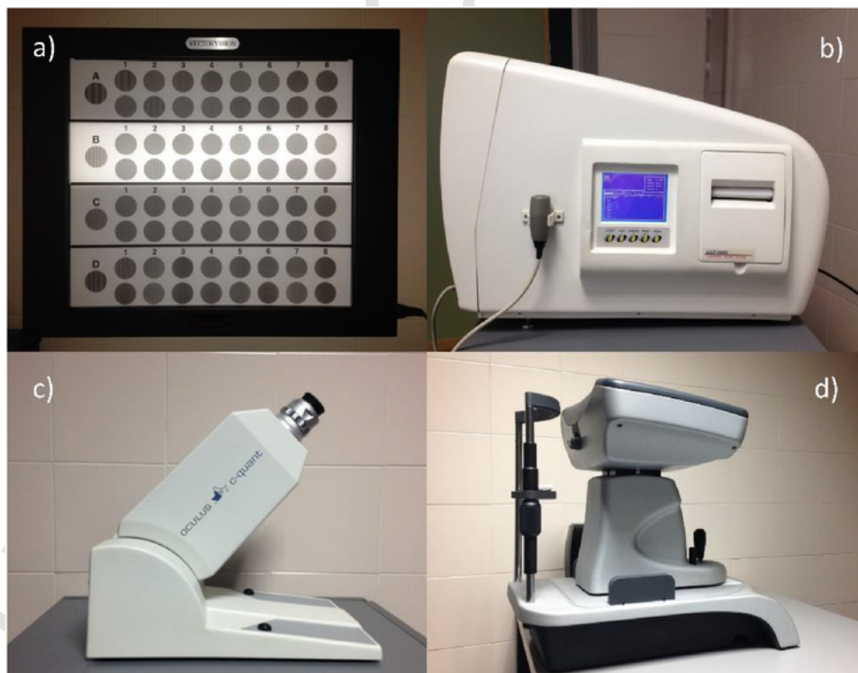
Fig. 1. Optical instruments used for evaluating visual and optical performance: a) CSV-1000 test, b) CGT-1000 test, c) C-Quant meter, d) OQAS II device.
