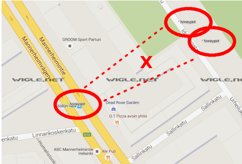
Figure 4.1: Circles show the information WiGLE has from a SSID called “honeypot”. The red X indicates the actual location of this access point.
