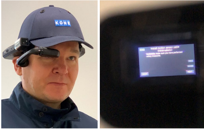
Figure 13: RealWear HMT-1 smart glasses (left) and their small screen (right)
