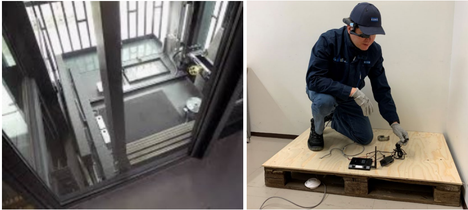
Figure 16: Real elevator car roof in elevator shaft (left) and elevator car roof simulation with pallet in meeting room
