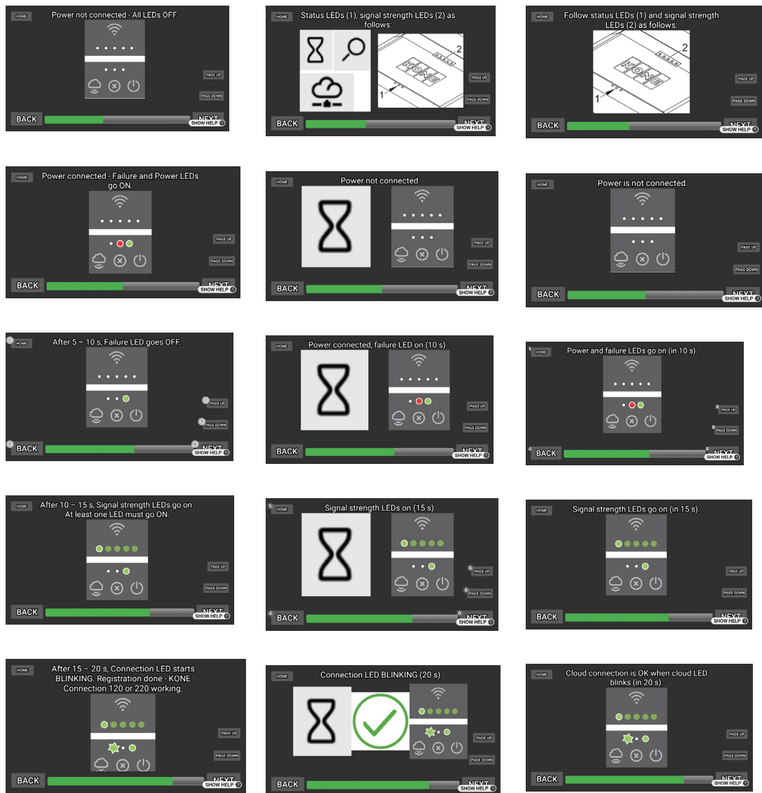
Figure 31 Steps 5 – 9 of “Power up KONE Connection”: conventional (left), visual manual (middle) and minimalistic (right)
