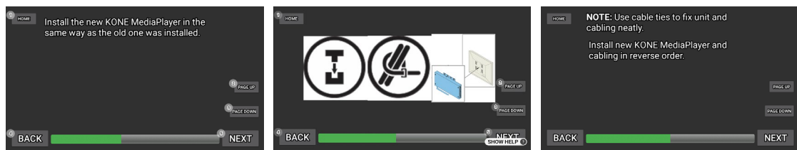
Figure 40 Step 6 of “Replace KONE MediaPlayer”: conventional (left), visual manual (middle) and minimalistic (right)
