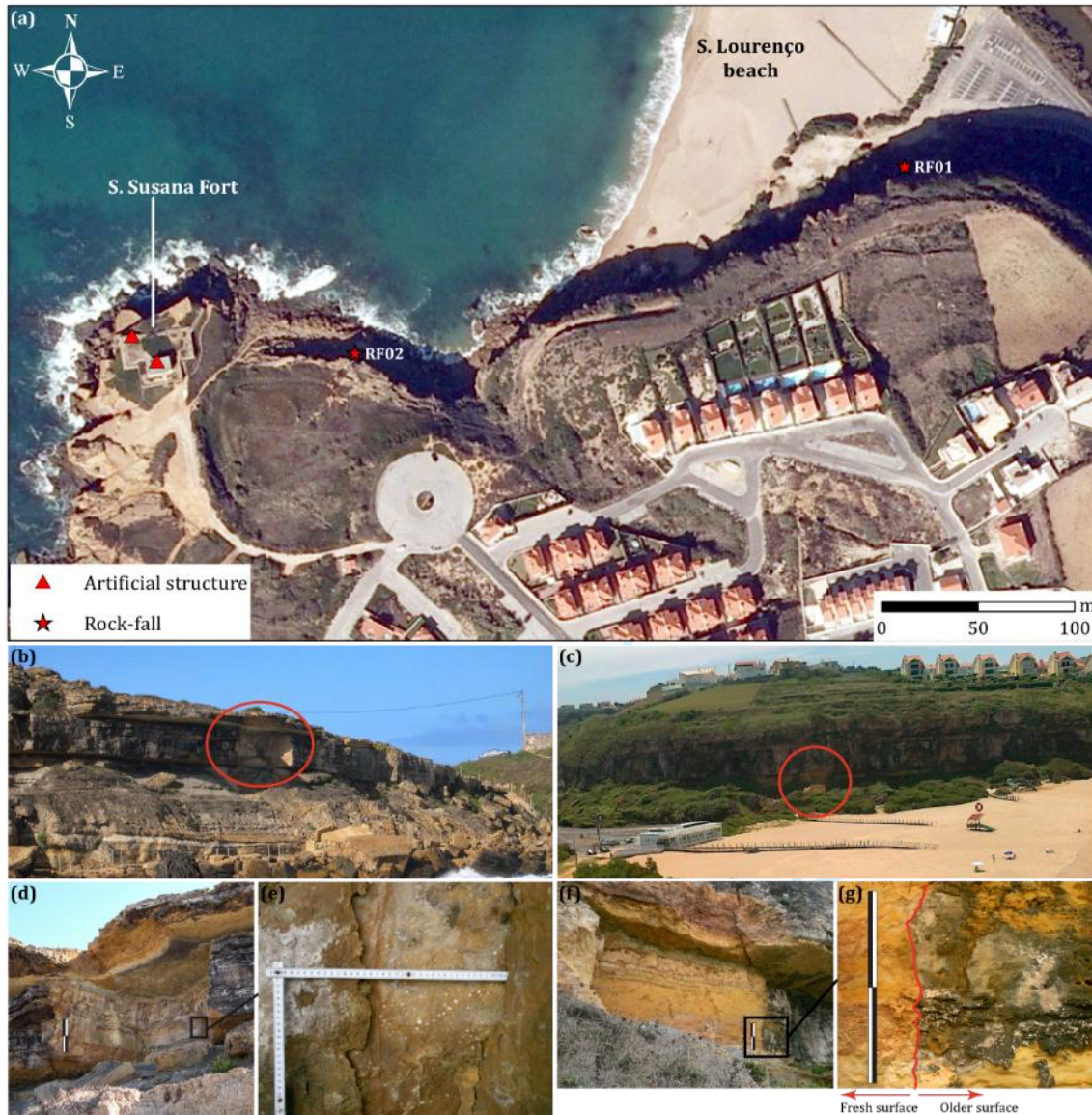
Figure S10: (a) Location of RF01 and RF02 control points over digital orthophotos (IGEO, 2010). (b) RF02 Rock-fall scar circled in red. (c) RF01 Rock-fall scar and resulting boulder circled in red. (d) RF02 rock-fall scar (vertical scale corresponds to 1m). (e) Detail of lichen cover in RF02 (vertical scale is 0.2m, and the horizontal scale is 0.4m). (f) Part of RF01 surface. (g) Detail of the contrast in lichen cover between the RF01 fresh and older surfaces (vertical scale corresponds to 1m).
