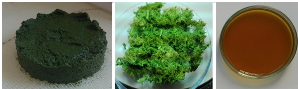
Figure 1: Alfalfa green biomass originated fractions: leaf protein concentrate (LPC), green fibre, brown juice Source: Own construction based on Kovács Z. (2020)
