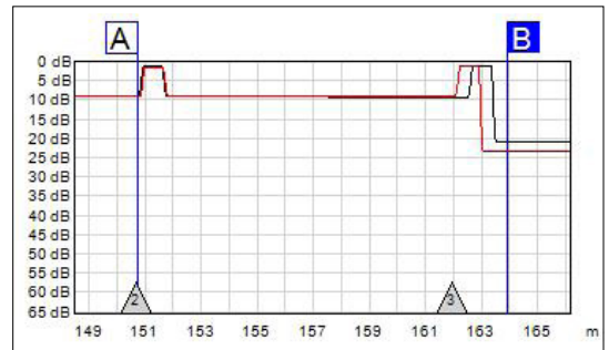
Figure 14. A detail of the OTDR measurement graph of the fiber loaded in the two gripped specimens.
