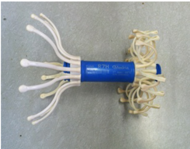
Fig. 1. Intra-vaginal thermometer (11.5 cm × 2.2 cm) used for multiparous cows.
