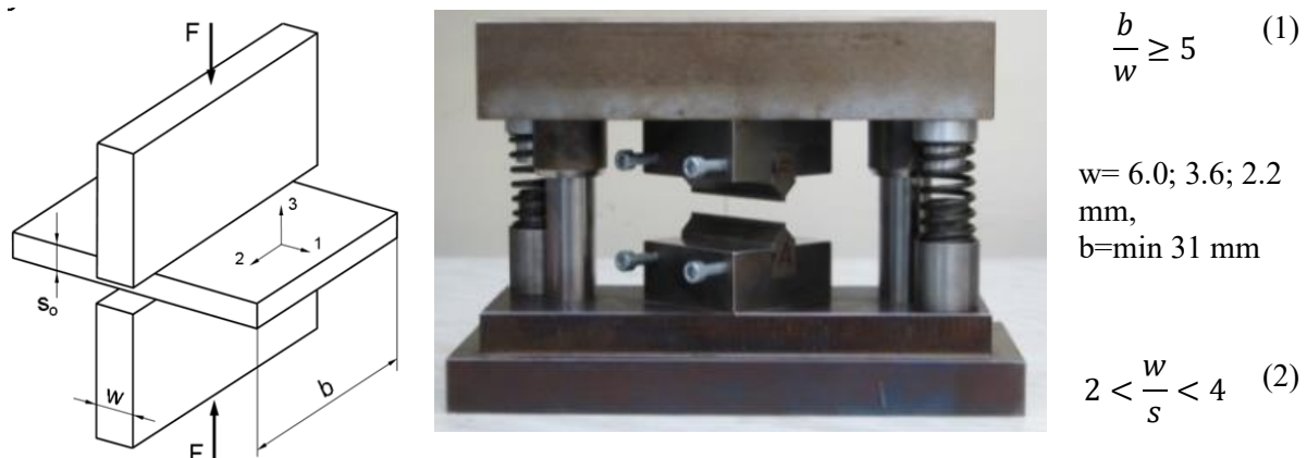
Figure 3. Geometry for Watts-Ford test ( s_0 – initial thickness of specimen, b – initial length of specimen, w – width of dies, F - force) and the inserted die in holder
