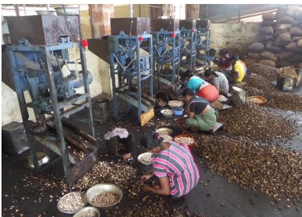
Photos 1-3 Semi-mechanised and manual cashew processing in India (Photos: J. Tessmann)
