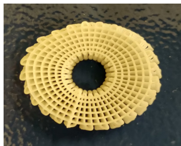
Figure 1: Example of bone brick produced using a 0/90° lay-down pattern and a pore size gradient (from 700µm to 300µm). The total porosity is 74%
