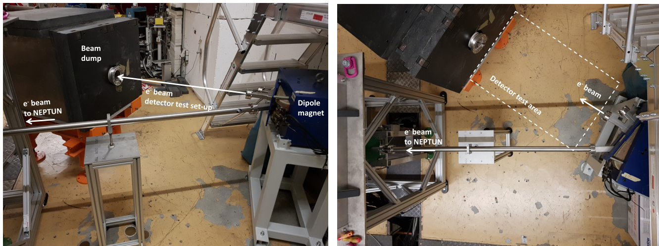
Figure 8.22.: Side (left) and top view (right) of the multi-purpose detector test set-up. Any kind of detectors can be placed between the dipole chamber exit window and the beam dump.
