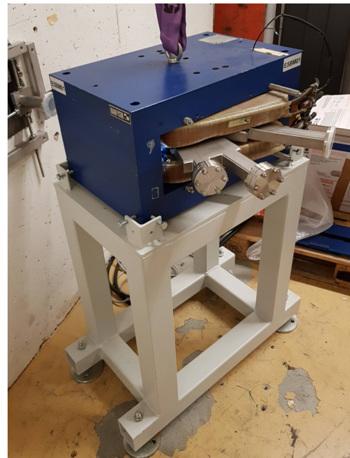
Figure 8.18.: Schematic drawing (left) and photograph (right) of the support structure for the dipole magnet. The construction allows an alignment of the dipole with the help of several adjustment screws. Detailed technical drawings of all sub parts can be found in Appendix A.2-A.6.
