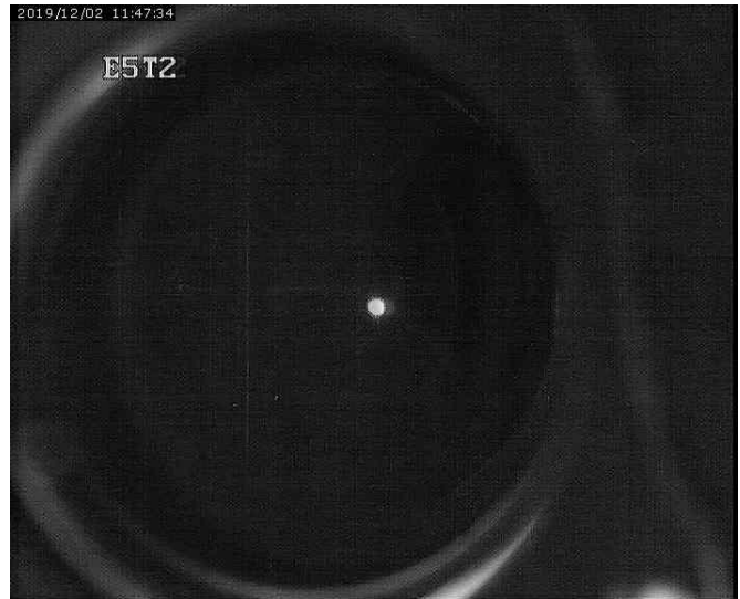
Figure 8.28.: Left: Camera picture of the E5T2 target which is located in front of the NEPTUN radiator. One tick is 5 mm, one pixel is 5/55 mm. Right: Beam spot on the same target without external illumination.
