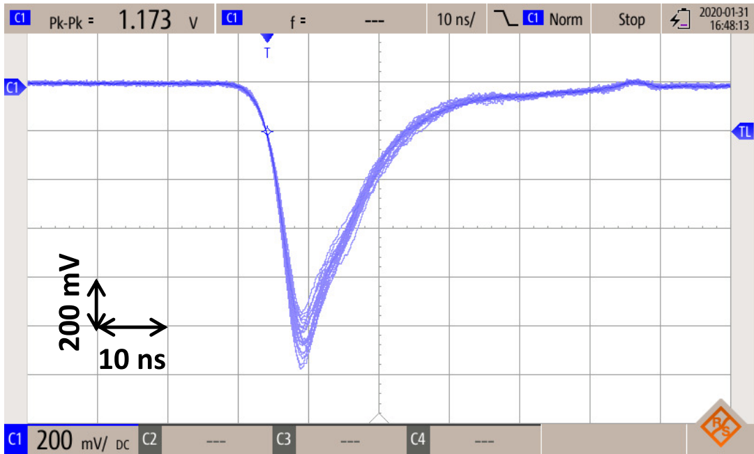
Figure 2.9.: Raw signals of an ECAL module containing a 3-inch Hamamatsu R6091 PMT. The signals are generated by LASER light, which is coupled into the lead glass.
