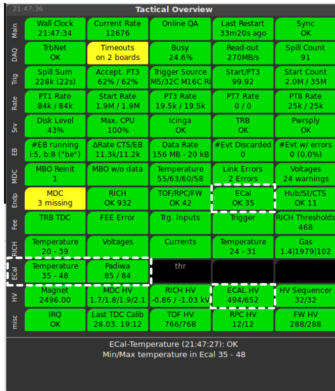
Figure 5.12.: The central monitoring tool in HADES is the tactical overview which visualizes the current status of the sub detectors and the DAQ-system using a simple color code. The most important parts for the ECAL operator are marked, e.g. the indication that all TRB3sc and PaDiWa-AMPS2 boards are addressable, the temperature of the boards and the state of the high-voltage system.
