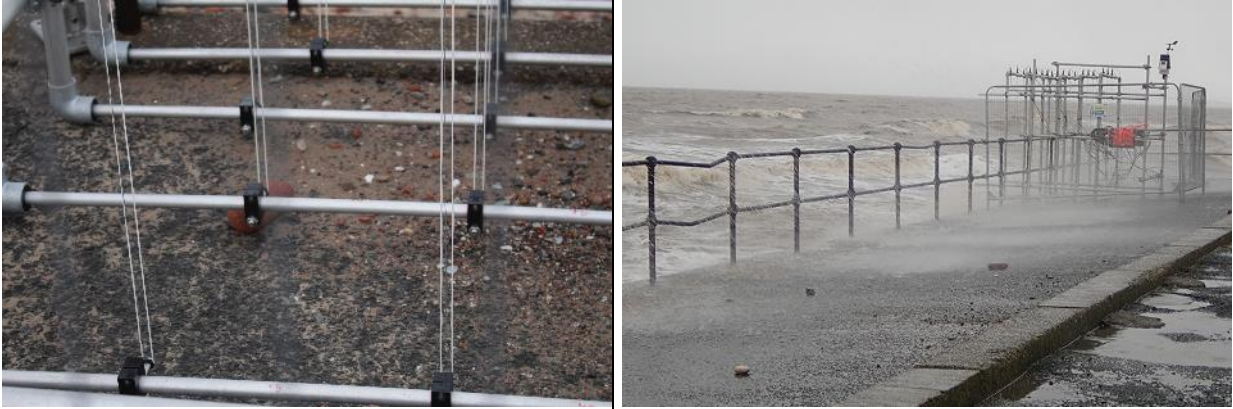
Figure AIII.10: Example of debris overtopping the wall during WireWall deployments. Debris found on arrival at site morning of the 8 th November 2018 (left). Brick debris overtopping south of the rig during on the 22 nd January 2019 (right).
