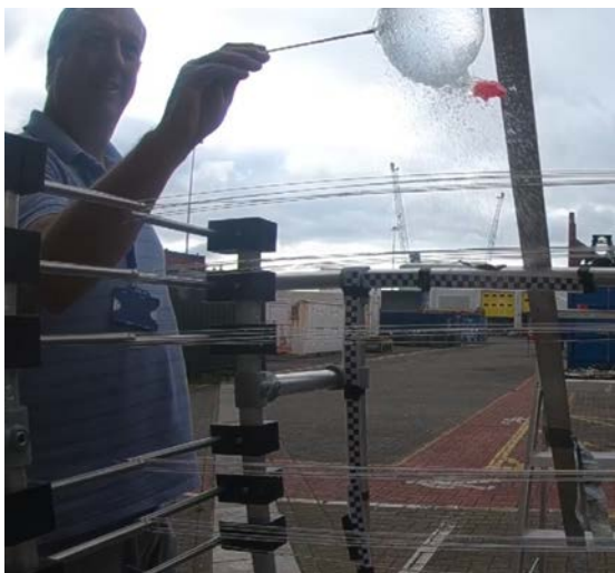
Figure 3.4: Top: schematic showing how the changes in measured depth and speed for a flow at an angle to the horizontal (red) offset each other and produce the same volume as the actual depth and speed of the flow (green). Bottom: balloon tests to validate speed measurements. The wires are now oriented
