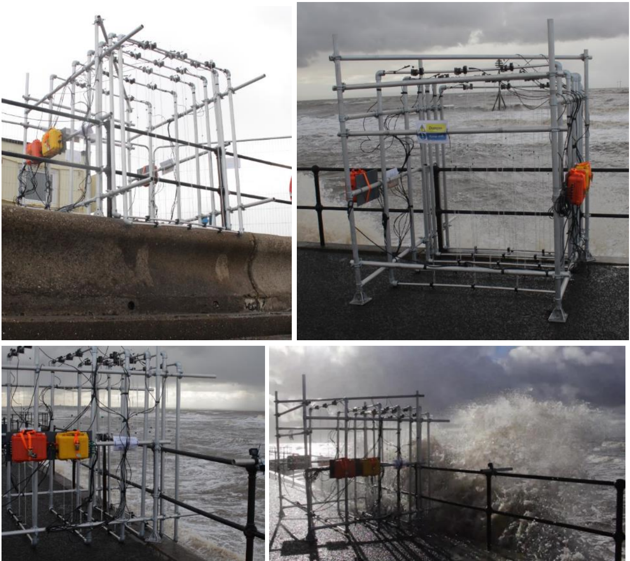
Figure 3.10: The first WireWall field deployment with overtopping examples taken during high tide on the 26 th October 2019.
