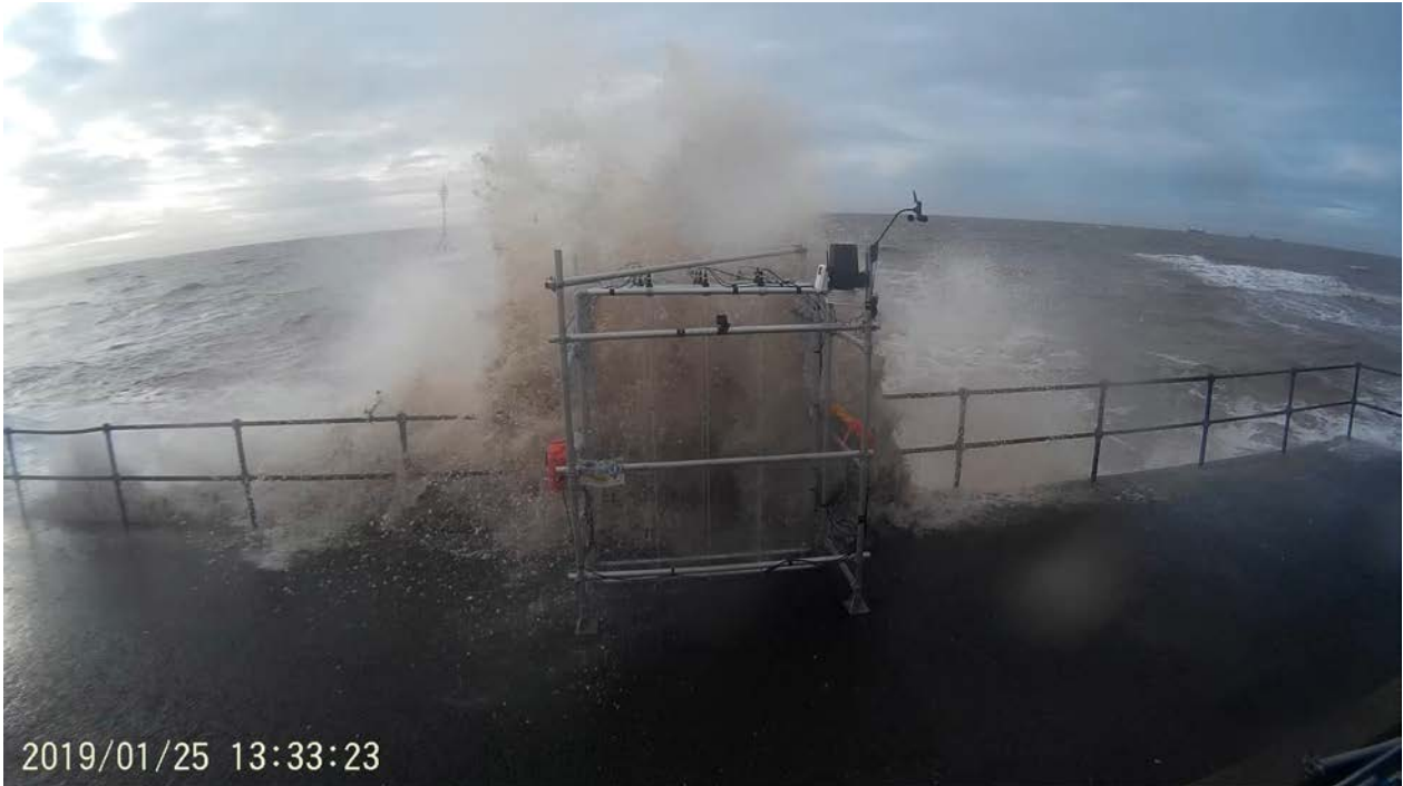
Figure 4.23: Still image of one of the very largest plumes observed during the deployment on Friday 25 th January 2019. It can be seen that the seawards part of the plume is taller than the rig. However, the upper part of the plume is made up of quite fine spray compared to the much denser spray/solid water lower down. In addition, the height of the plume reduces as it travels through the rig.
