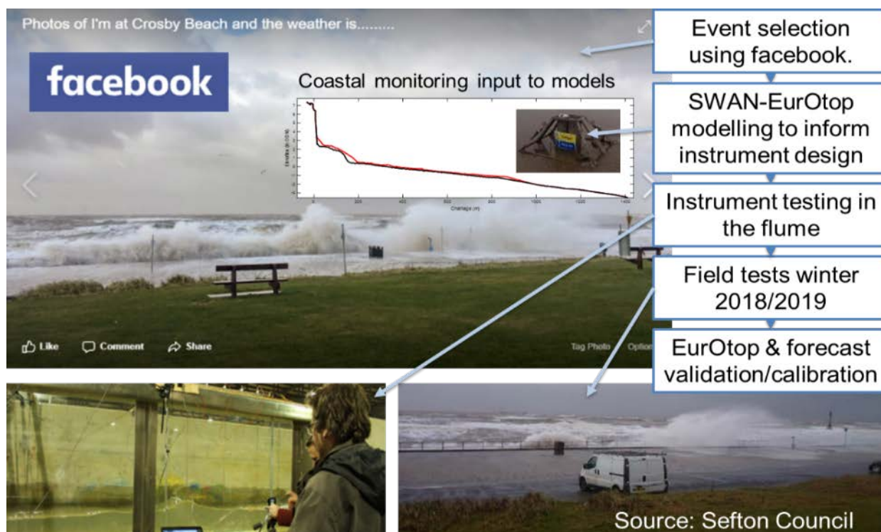
Figure 1.2: The WireWall approach to collect new observations required to identify site-specific safety thresholds & calibrate models used in scheme design.
